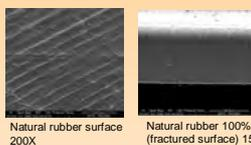
**Homogeneous** in mass with teflon mold marks on surface.
